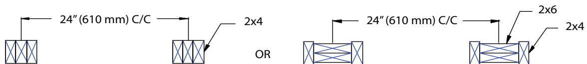
Figure 2: Support wall configuration
